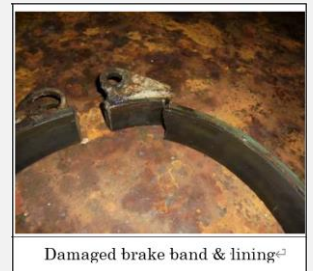
Damaged brake band & lining ©
