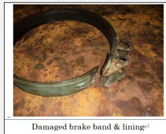
Damaged brake band & lining ©
